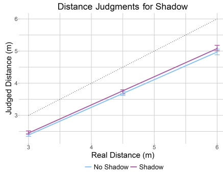
Figure 5: Judged distance vs. real distance for each shadow condition fit with linear regression. The solid lines represent performance for the shadow and no shadow conditions, while the dotted line represents veridical performance. Error bars are \pm 1 standard error.
