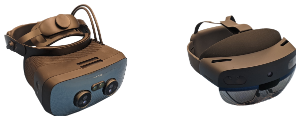
Figure 1: The Varjo XR-3 (left) is a video see-through (VST) augmented reality display. The HoloLens 2 (right) is an optical see-through augmented reality display.
